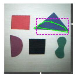
**Figures 5a and 5b.** Sample gaze-only results for Experiment 1. The eyetrace is shown in green; the hypothesized region of interest is shown as a dashed magenta box. Figure 5a (left) shows how the "box squashing" algorithm ameliorates the effects of noise spikes in the eyetrace. Figure 5b demonstrates that when the eyetrace is poor—here the subject has "short-cut" the top vertex of the triangle—the gaze-only algorithm can pay dearly for ignoring boundaries in the image itself.
