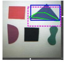
**Figure 8.** Sample fusion results for Experiment 1. Eyetraces are shown in green, the gaze-only solution is shown as a dashed magenta box, and the output of the fusion algorithm is in blue. Using the color structure of the images the fusion algorithm was able to overcome these inaccurate eyetraces to achieve an excellent solution.
